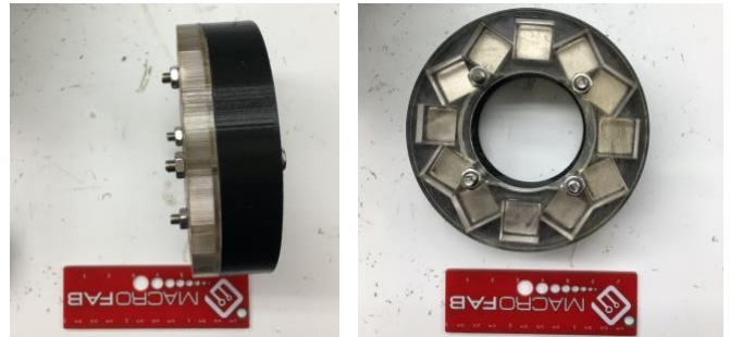
Fig. 37. Assembled halbach array used to create a homogenous magnetic field to prevent the magnetic particle from clustering or drifting.
