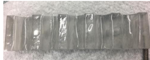
Fig. 24. Ecoflex film layed on the inner surface of one half of the mold
