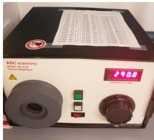
Fig. 38. ASC SCIENTIFIC impulse magnetizer (Model IM-10-30)
