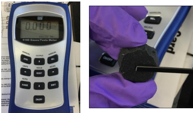
Fig. 39. F.W BELL 5180 Gauss/Tesla meter being used to characterize a fabricated magnetic sample made out of strontium ferrite and Ecoflex 30
