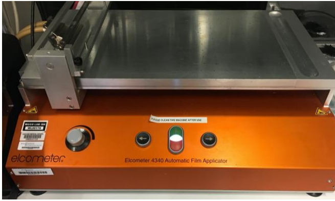
Fig. 21. Elcometer 4340 Automatic Film Applicator is used to create a thin layer of Ecoflex that is then used to make a shell to contain iron particles.
