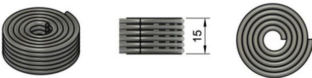
Fig. 11. CAD of the flexible soft coil with 30 turns and 10 mm diameter
